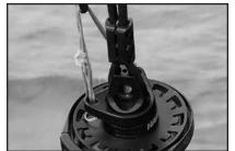
**7356 fairlead kit** - For cruising, lead the furling line loop back to the cockpit. Leads fit 25 mm (1") stanchions. Includes two double fairleads, a double fairlead with cleats, and aft block with bungee.
