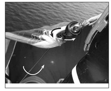
When furling an asymmetric spinnaker, the sail tack is on a swivel and does not begin furling until most of the sail is furled. When furling a code zero sail, the sail tack is fixed.
