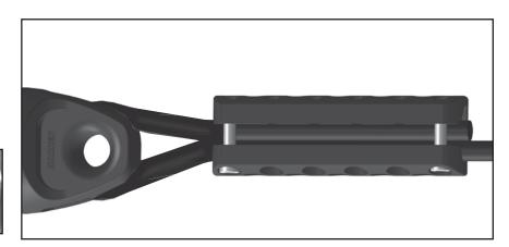
4. Push the clamp assembly toward the thimble. Squeeze the torsion cable at the thimble. Position clamp about 20 mm (3/4") from the thimble. Leave a tail beyond the clamp.
