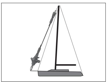
IMPORTANT! After sailing with the cable for the first time in significant wind, retighten all screws in upper and lower cable clamps. The clamp halves should close together. Use a torque setting of about 40 Nm (30 ft-lb).
