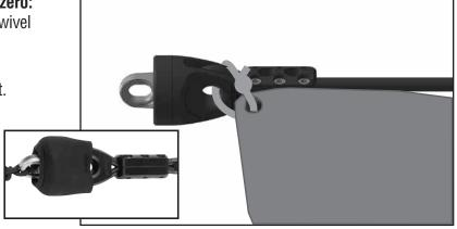
**Securing tack**, **asymmetric spinnaker**: Secure tack of sail using soft-attach long shackle secured to the tack swivel. Make length adjustable for adjustment when sail is finally fitted.
