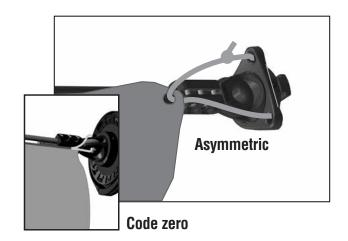
Load the Reflex tack terminal into the T-slot on the lower drive unit. Attach the unit to the bow sprit or a fixed point on the bow ahead of the stay. Attach halyard to head swivel and check halyard and sheet leads. Hoist and trim spinnaker.
