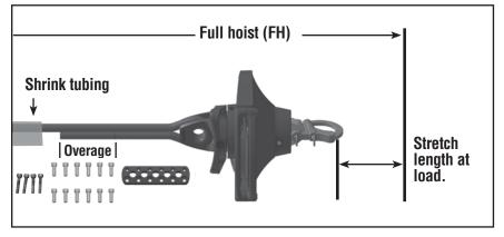
**6. Building the tack terminal:** Follow the procedure used to build the head swivel terminal from pages 10 and 11.
