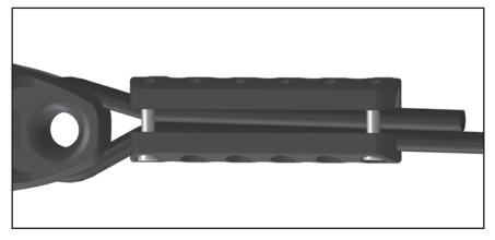
IMPORTANT! - Secure the torsion cable to the head swivel first. Wait to cut the torsion cable to length until you can check the length by dry-fitting into the assembled drive unit with tack swivel and threaded adapter in place.
