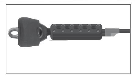
10. If assembling away from the boat, lay cable out straight. Install tack terminal and snap shackle adapter on drive unit. **Note:** See following pages for preferred method of determining length at boat.
