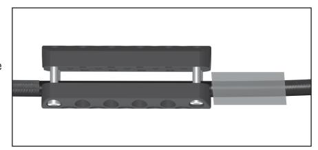
3. Insert the end of the cable through thimble at the head swivel and position it at the desired location on the cable. Slide the clamp assembly over the end of the cable as shown. *Tip: Secure the head swivel in a vise when building the terminal to hold it in place.*
