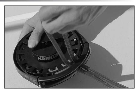
Work the line into the space between the drive sheave and the flexible cowling.
