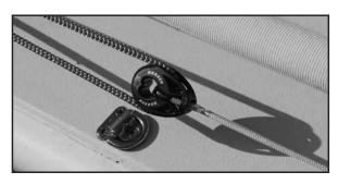
**Installing continuous furling line loop:** Follow instructions in manual to load the furling line into the furler. Load the line into the fairleads by bending into the openings. Push the line into place.
