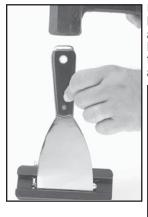
Use a thin flat device like a putty knife and use a small hammer to lightly tap slider into car as far as it will go.
