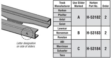
Start by slipping slider on side overhangs of "T" part of track. Slider should fit easily without too much play. To further check fit, slip inserts length-wise into one end of car about 1" (25mm) until tabs stop them. Slide car with partially inserted inserts onto end of track.
