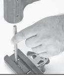
Once slider is in channel, use a rod or screwdriver and tap the bosses into the recess on underside of car.
